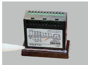
Figure 5: Apply silicone around the frame as shown.
