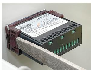
**Figure 8:** With one hand pressing firmly on the face of the controller, use a file or similar item to push the ratchet clips and tighten the seal.
