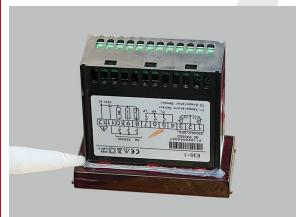
**Figure 5:** Apply silicone around the frame as shown.
