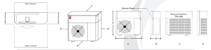
Note: 8G R32 Series heat pumps and chillers are not suitable for indoor/plant room installations without air quality monitoring and ventilation due to mild flammability.
