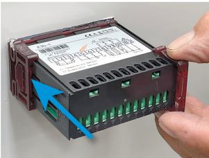
Figure 7: With one hand pressing firmly on the face of the controller, push the ratchet clips and tighten the seal.
